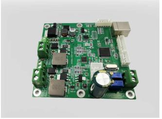
**OEHTC-200 Heater Temperature Controller (OEM)**
